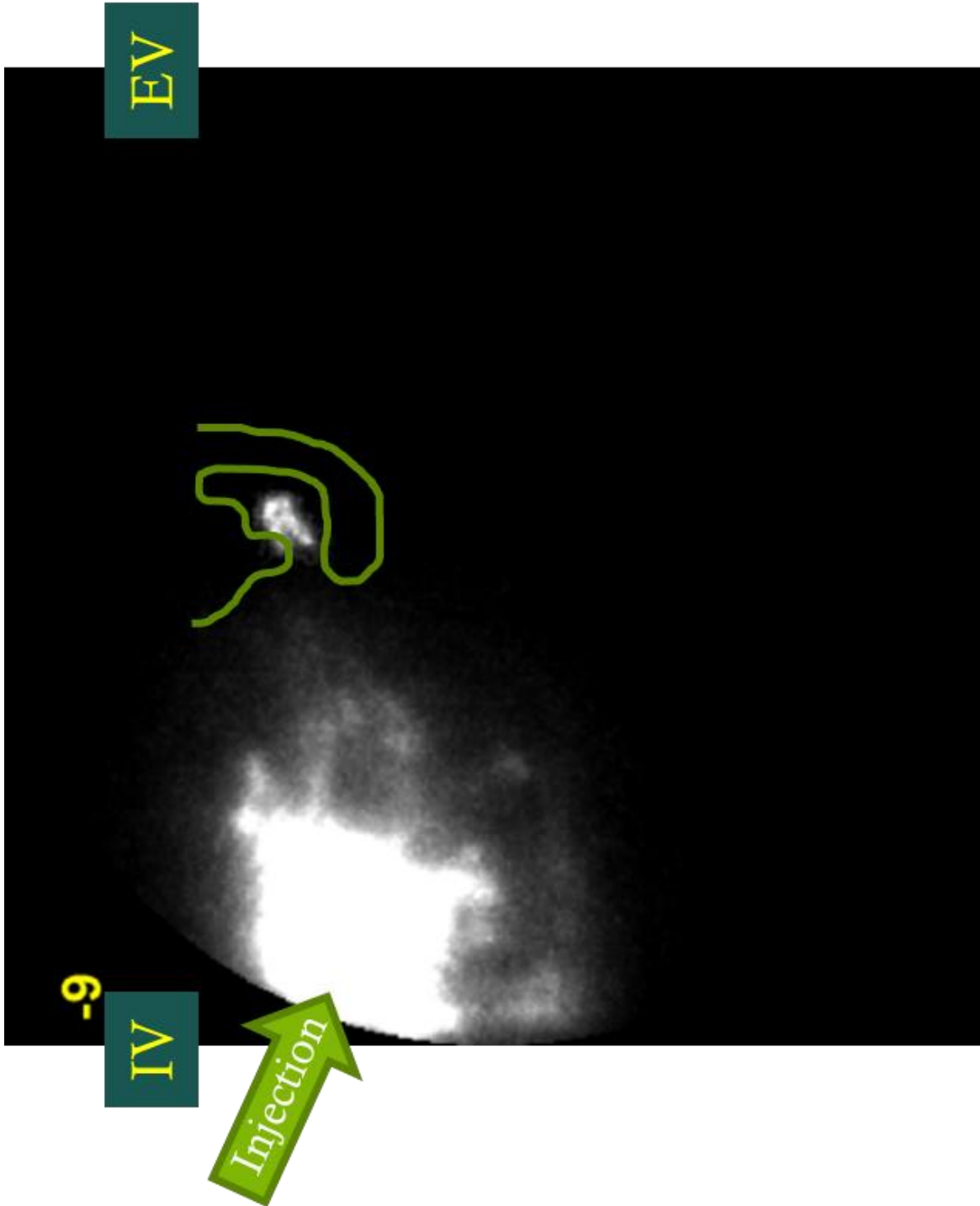
Figure 4.8.5 (b) Pre-ignition image (1° after ST)
