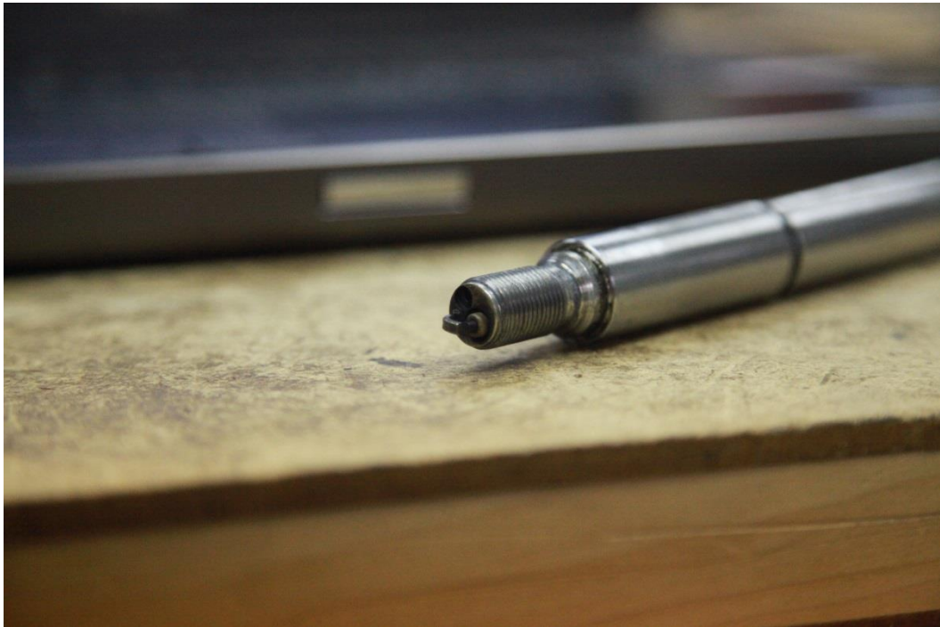
Figure 3.2.3 (b) sOAE devices: in-spark-plug pressure transducer
