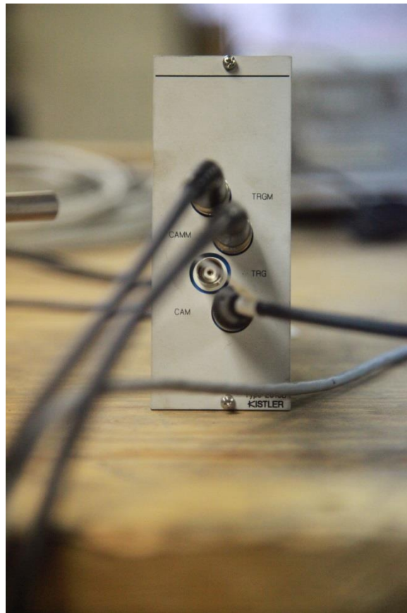
Figure 3.2.4 (d) mOAE devices: Kistler 2613B encoder (top) and its outputs (bottom)
